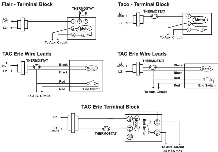
Figure-3 Typical Wiring of a PopTop to Replace a Flair or Taco 3-Wire Valve.
